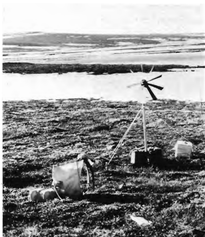
Figure 4. The wind generator in operation, trickle charging uninsulated six volt batteries, North Henik Lake, District of Keewatin.
