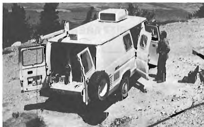
Figure 30.5. Logging a mineral hole near Ely, Nevada. The computer controlled data acquisition system is in the van. The draw work contains 3000 feet (about 1000 m) of cable. Electric power is supplied by a 5 kw gasoline power generator which is installed in the van.
