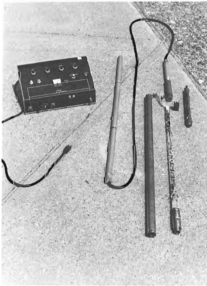
Figure 14.2. The T/R unit, a pole-dipole electrode array, and the disassembled logging tool showing circuit board containing amplifier, filter and V/F converter. Battery pack is shown with one of the three 9V transistor batteries beside it.
