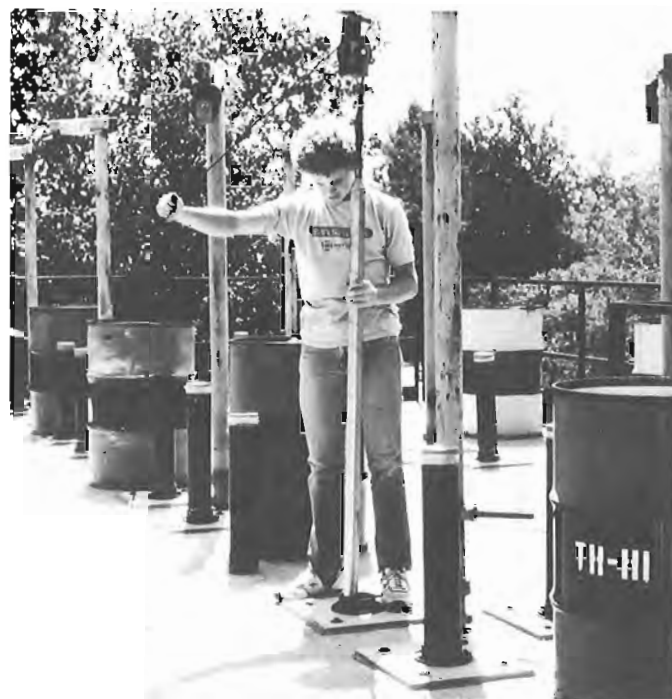
Figure 3.14. Lowering a gamma ray spectral logging probe into one of the model boreholes at Bells Corners. This view of the working area shows the overhead pulley assemblies, the black plastic extension pipes for aligning the probes with the holes in the model below (as well as permitting calibration when snow covers the work area), and the storage drums for antifreeze used in the boreholes. (GSC 202942-R.)
