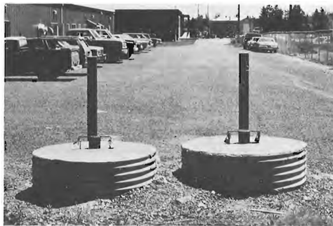
Figure 3.19. The four model boreholes located in Saskatoon, Saskatchewan, designed for calibration of gamma ray logging tools. They nominally contain: BU-1-S, 0.01% U; BU-2-S, 0.1% U; BU-3-S, 1.0% U; and BU-4-S, 4.0% U. (GSC 202942-Q.)
