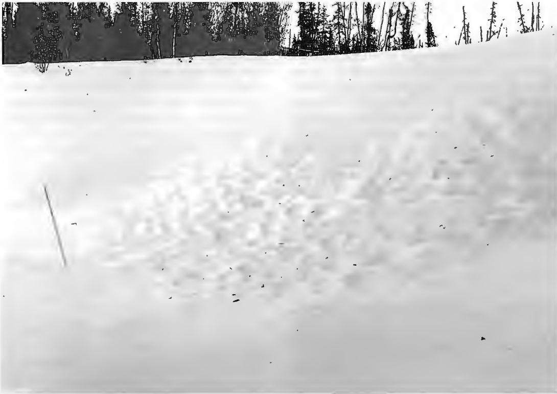
Figure 7. Hot spot, slope 45, October 1992. Hummocky, melting wet snow indicates high surface temperature in wood chips.
