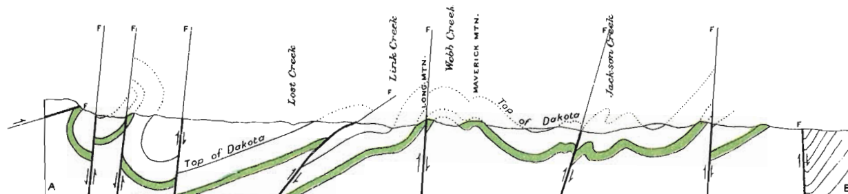
Diagrammatic structural section along line AB Scale, horizontal and vertical 15,840 feet to 1 inch
