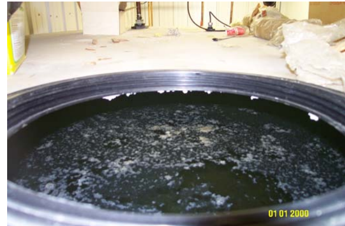
Photo 0105: 1950 Scum on Surface of Well Water Storage Tank
