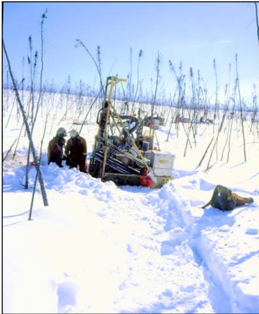
Figure 2.13: Winter exploration in Eagle Plains: setting up a portable drilling rig. (Photo: Yukon Energy, Mines, and Resources)
