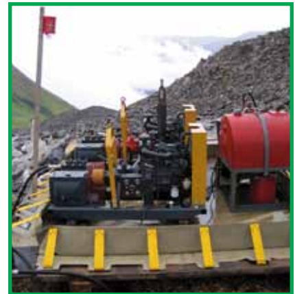
Mechanical equipment placed in an impermeable liner resistant to the product being used to collect drips and spills.
