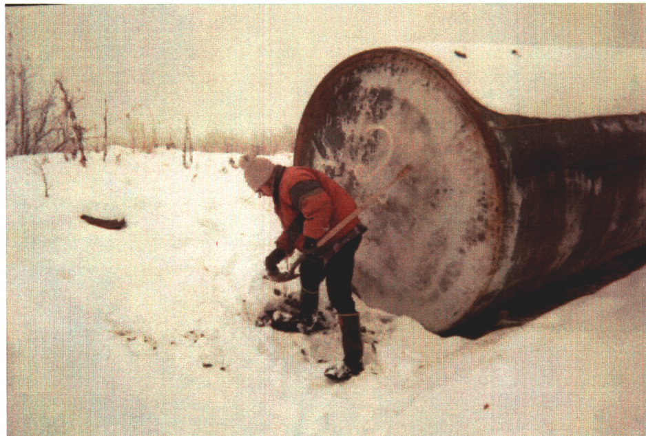
Photograph 27: Soil sampling at fuel tank # 2 showing earthen berm in background
