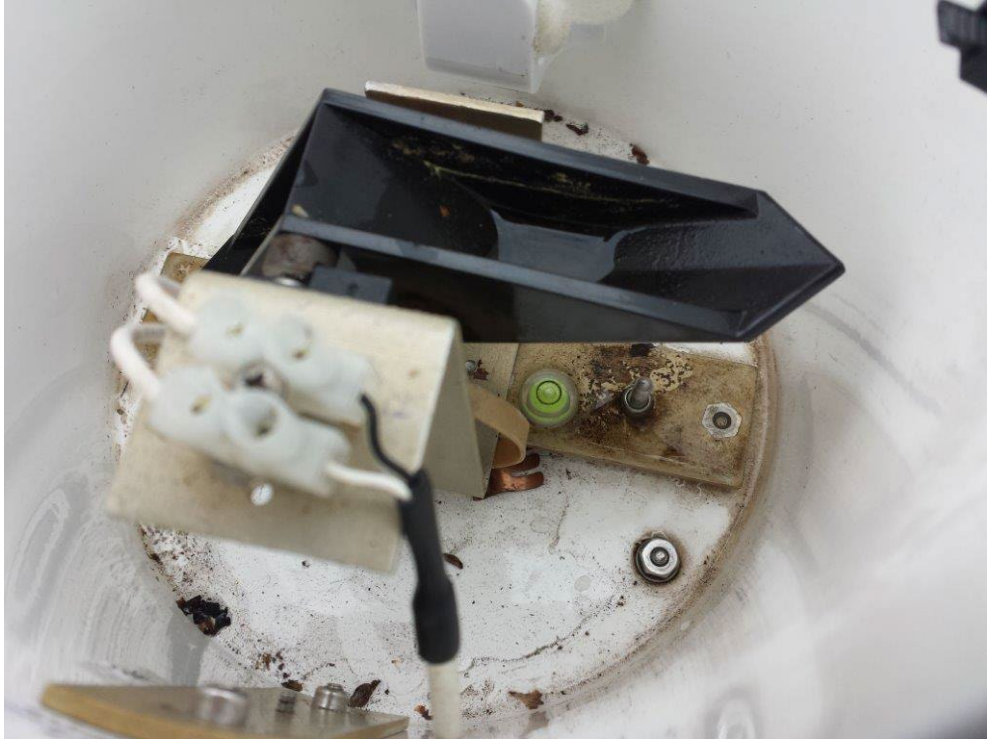
Figure 3 Levelling Bubble at Base of Tipping Bucket
