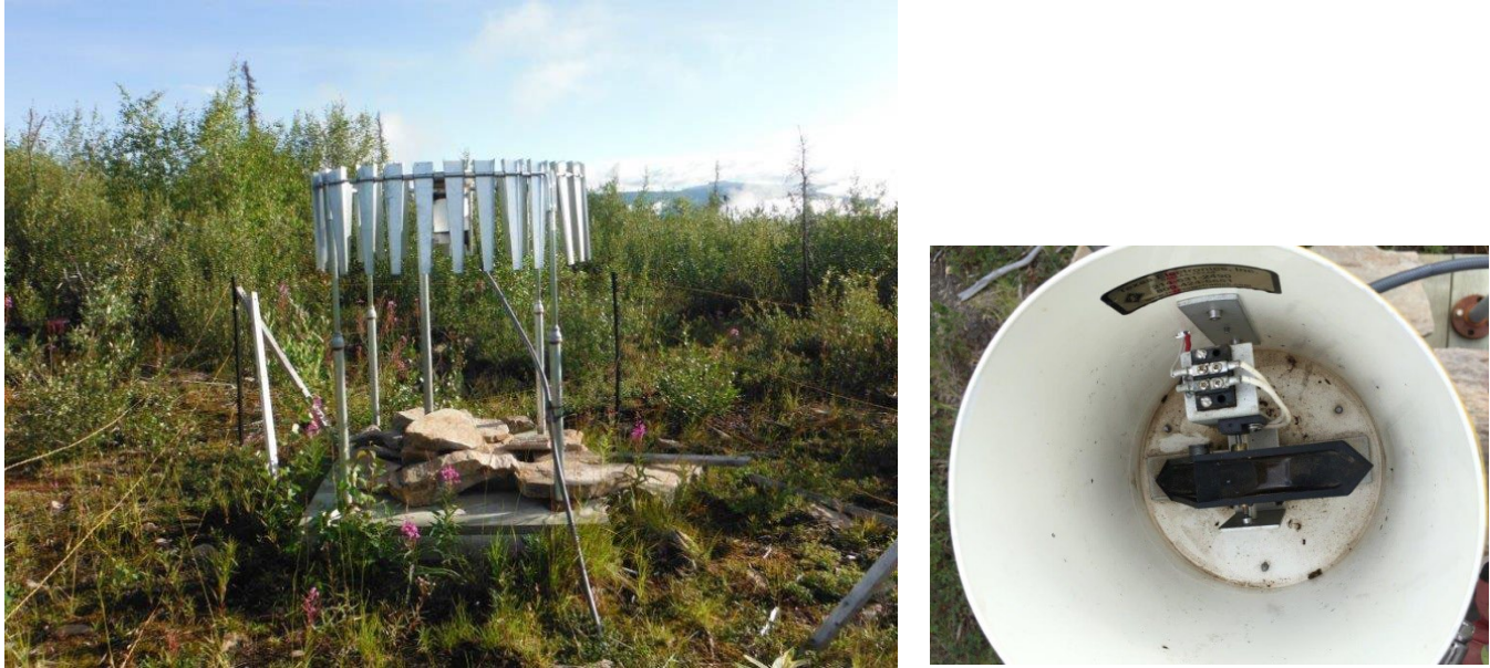
Figure 6 Precipitation gauge wind screen and plan view of tipping bucket
