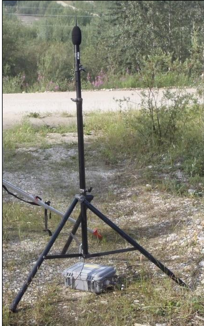
Figure 3-1 Larson Davis 831 Noise Meter Installed in an Environmental Enclosure with Microphone and Wind Screen
