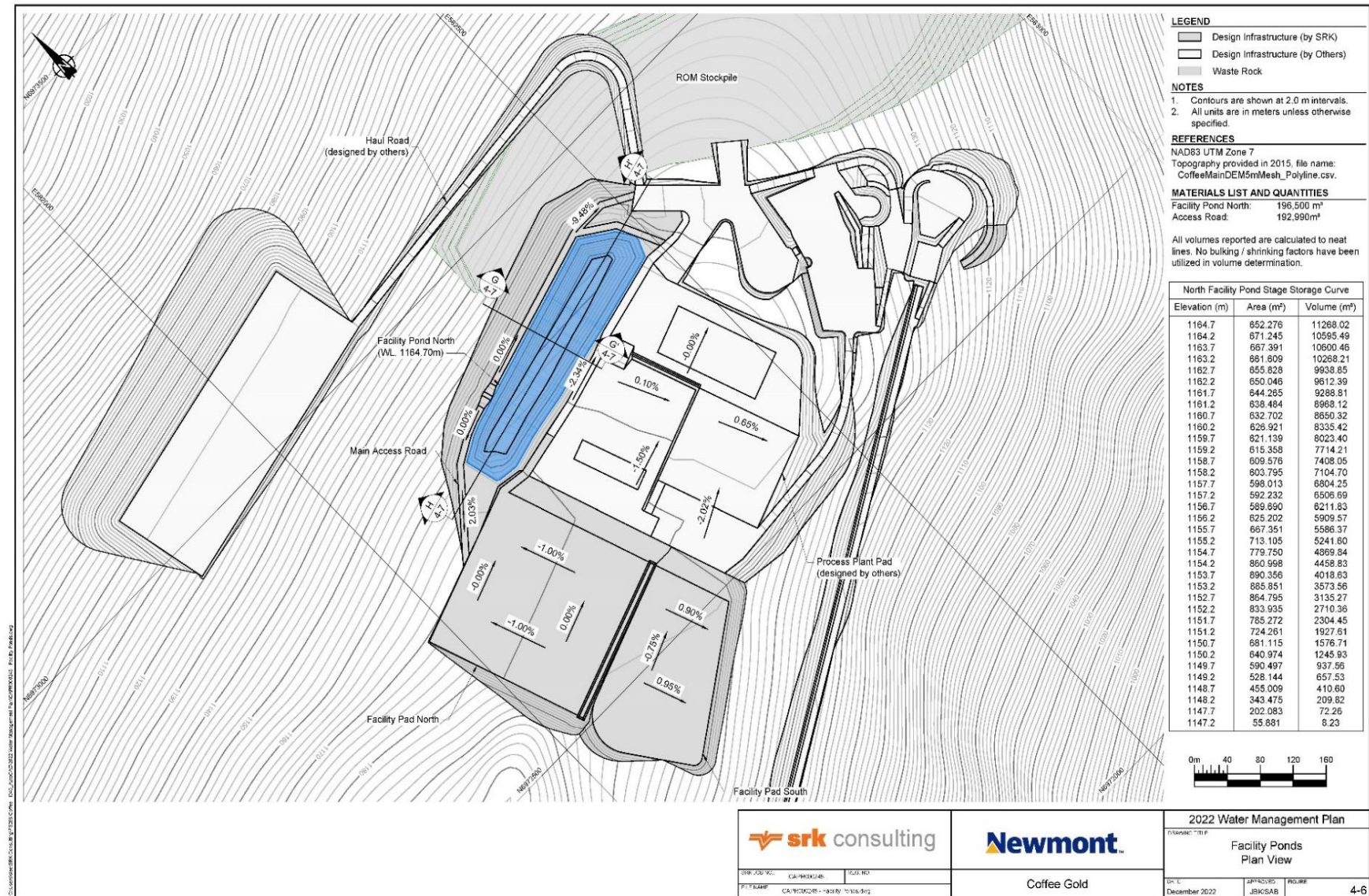
Figure 4-6 Facility Pond Detail Layout
