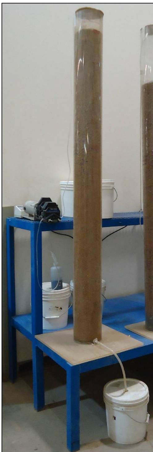
Figure 6-2. Eagle Gold Project Column Leach Test Apparatus
