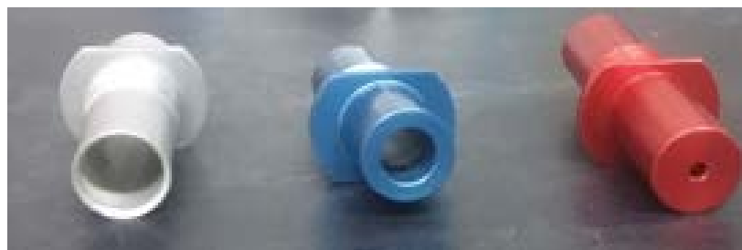
Figure 3 Inlet jet sizes: TSP (grey), PM10 (blue), and PM2.5 (red)
