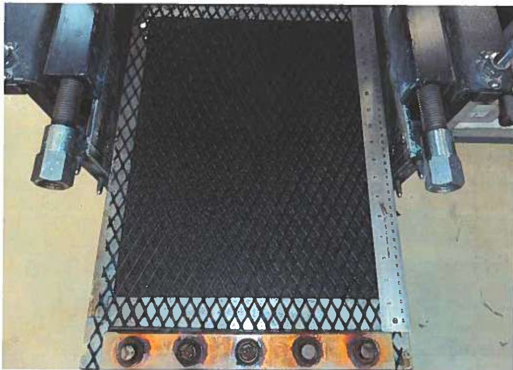
Geonet after the test – Test at 100kPa
