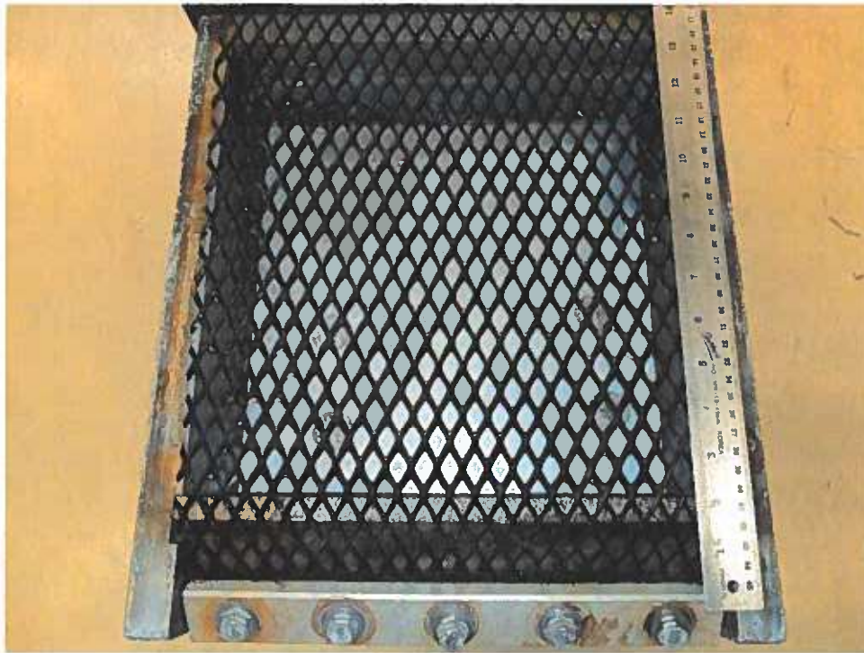
Geonet Hydranet 220 after the test - Test at 100kPa
