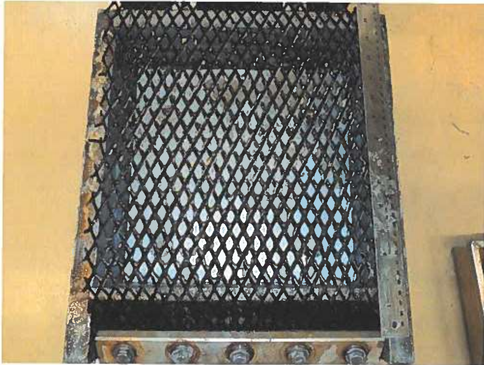
Geonet Hydranet 220 after the test - Test at 400kPa
