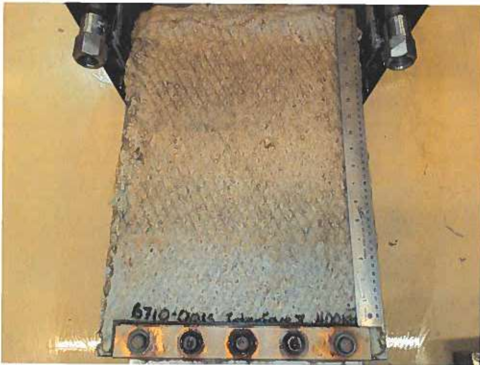
GCL Bentomat ST#10 (non-woven side) after the test – Test at 400kPa
