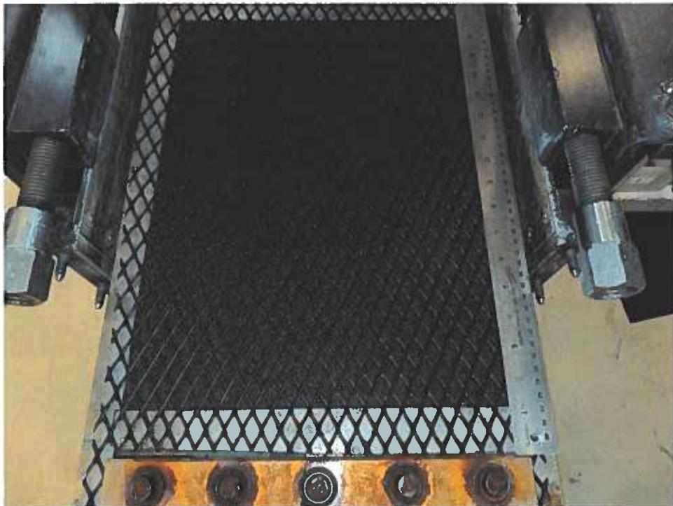
Geonet after the test – Test at 200kPa
