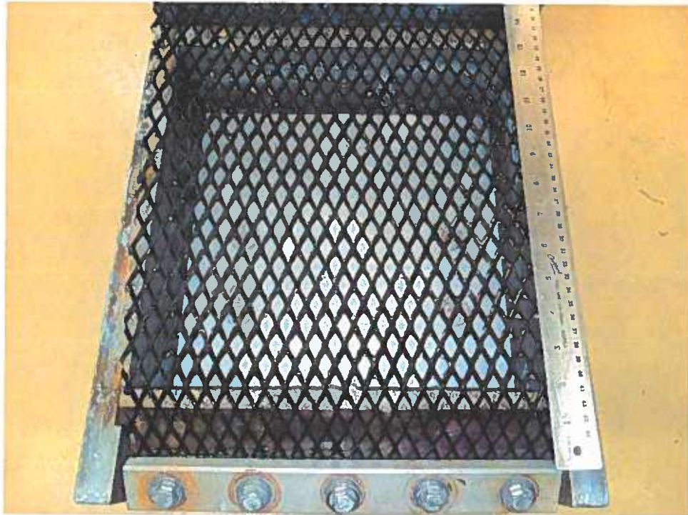
Geonet Hydranet 220 after the test - Test at 200kPa
