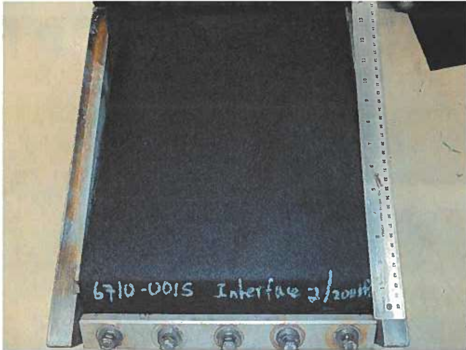
Non-woven Geotextile after the test – Test at 200kPa
