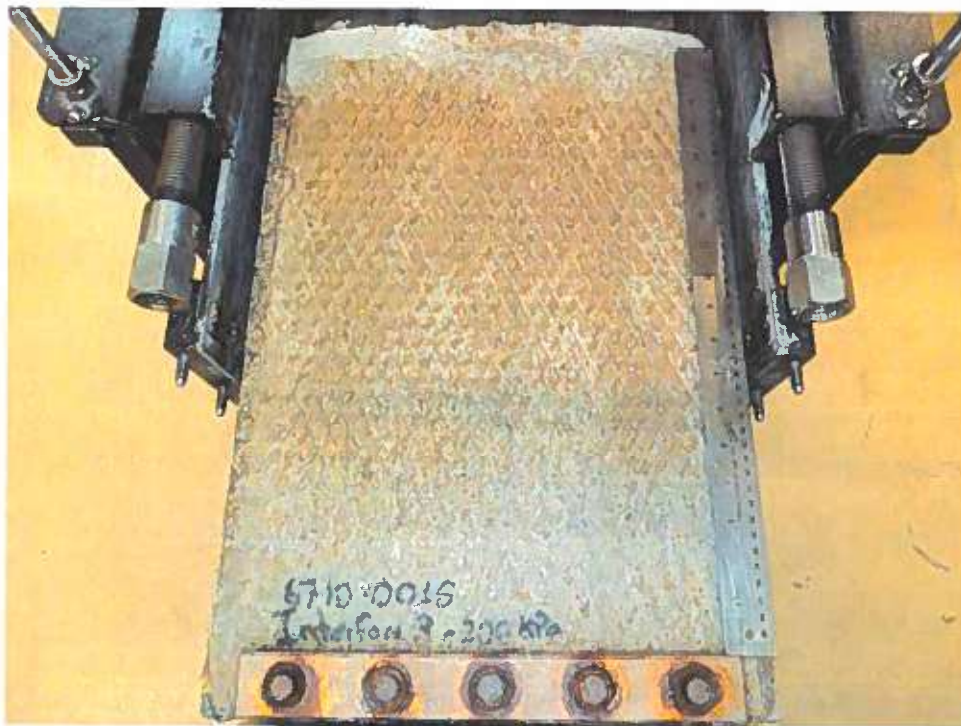
GCL Bentomat ST#10 (non-woven side) after the test – Test at 200kPa
