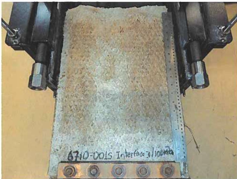
GCL Bentomat ST#10 (non-woven side) after the test – Test at 100kPa
