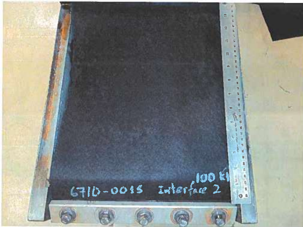
Non-woven Geotextile after the test – Test at 100kPa
