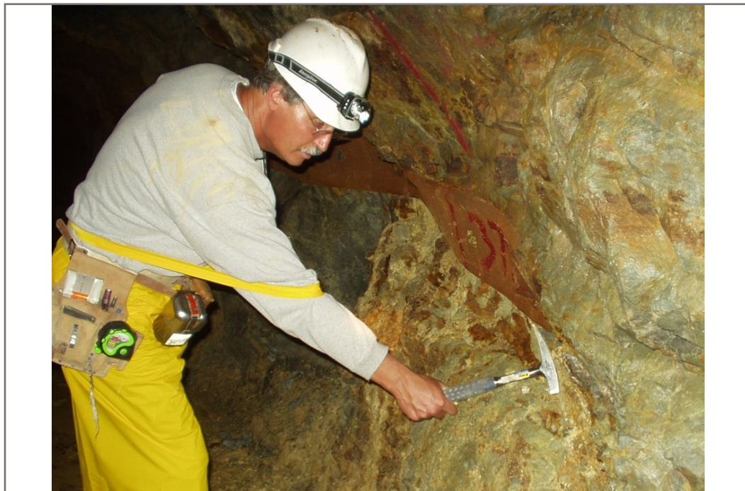
Photo 2: Geotechnical mapping of adit to determine plug site suitability. All ribs (walls) and back (roof) are to be removed of existing electrical and mechanical appurtenances, if present shall be removed from the plug footprint.
