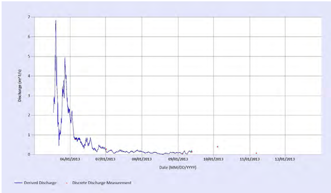
Figure C15 - Discharge at KV-9, Flat creek near the mouth, 2013
