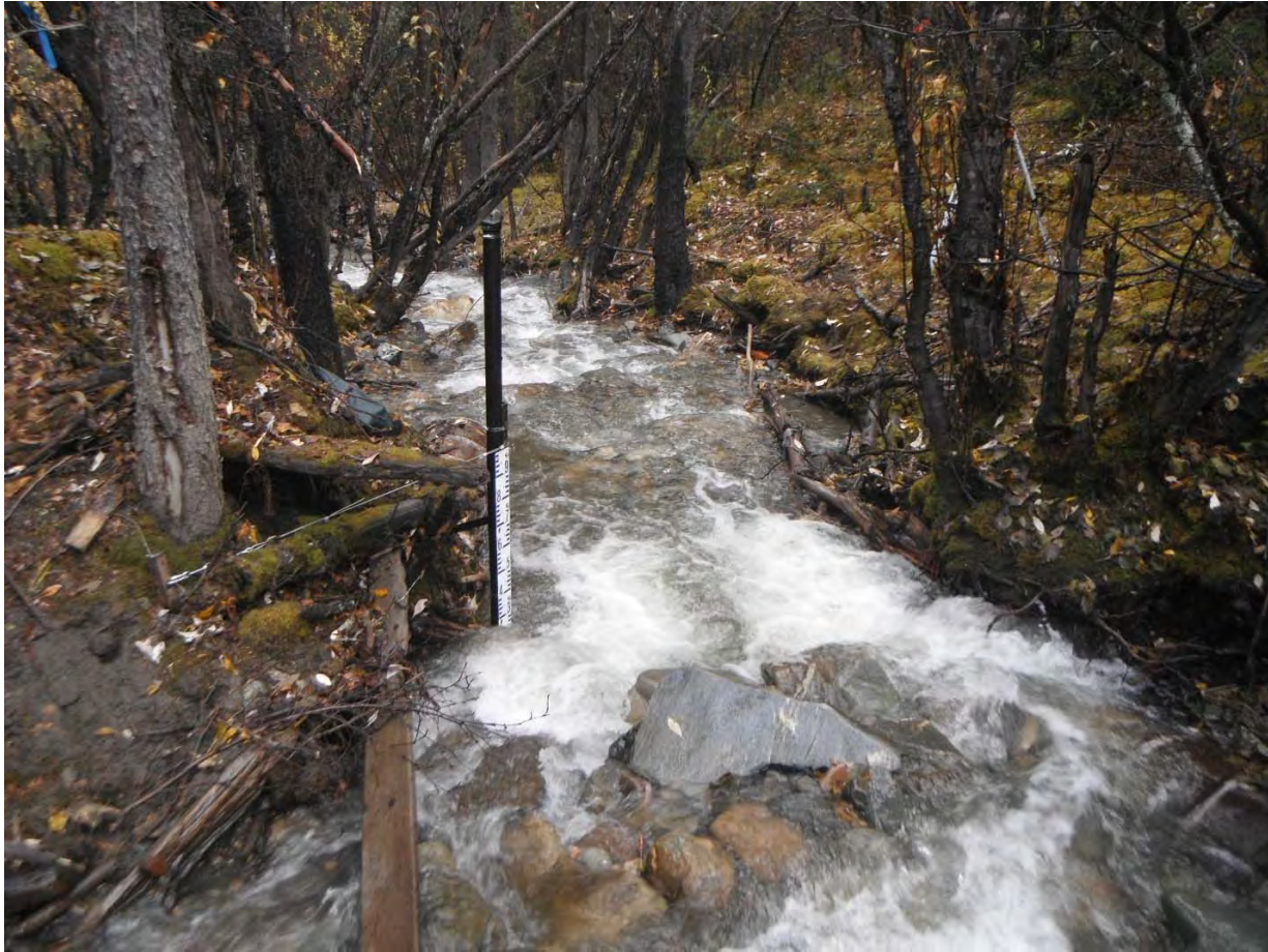
Figure 2 – KV-64 hydrometric monitoring station, installed in September 2015, below the Silver Trail Highway
