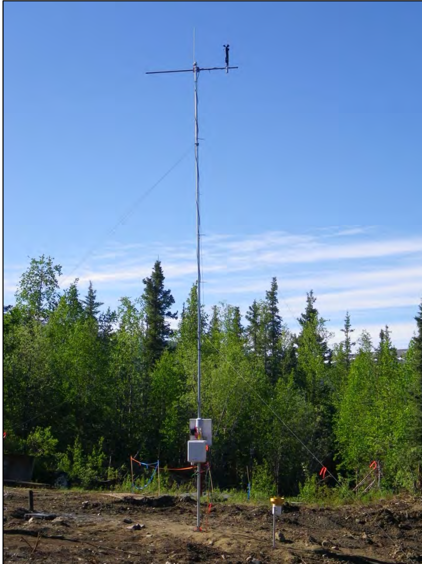
District Mill Campbell Scientific Meteorological Station
