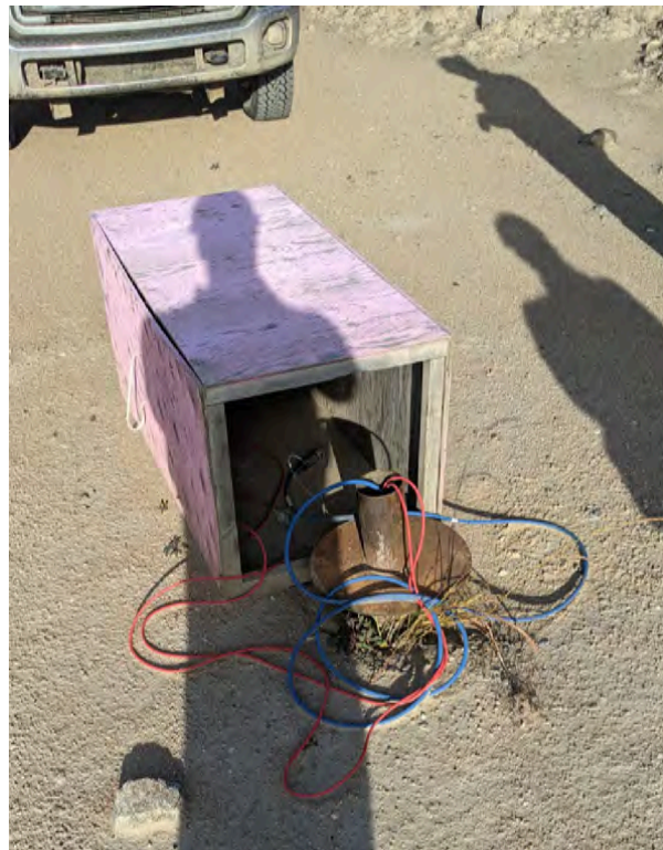
Photo 1-8: Piezometer DSP-06 and Thermistor DST-11 on the DSTSF waste rock crest. The instrumentation was found to be uncovered and exposed to the elements. Precipitation down the borehole could influence the instrumentation readings.
