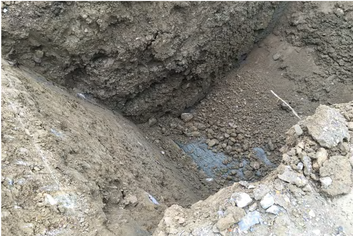
Photo 10: Test through the till cover on the tailings. Depth of cover about 2.14m
