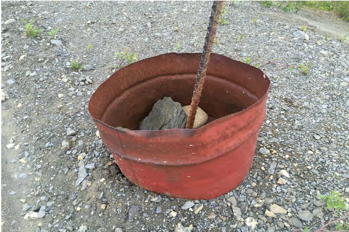
Photo 9: Deformation gauges installed during construction of the North Dam. Removed during decommissioning.
