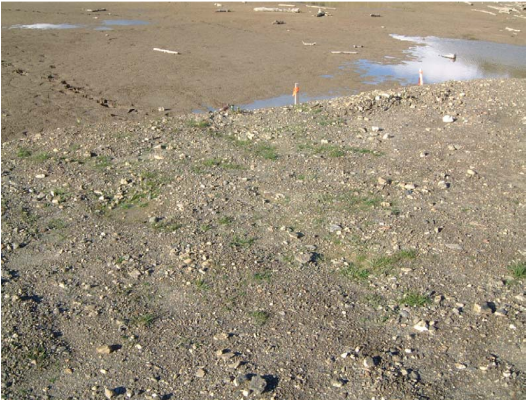
TMF with 500 mm rock and 300 mm soil – plot 2 in left foreground
