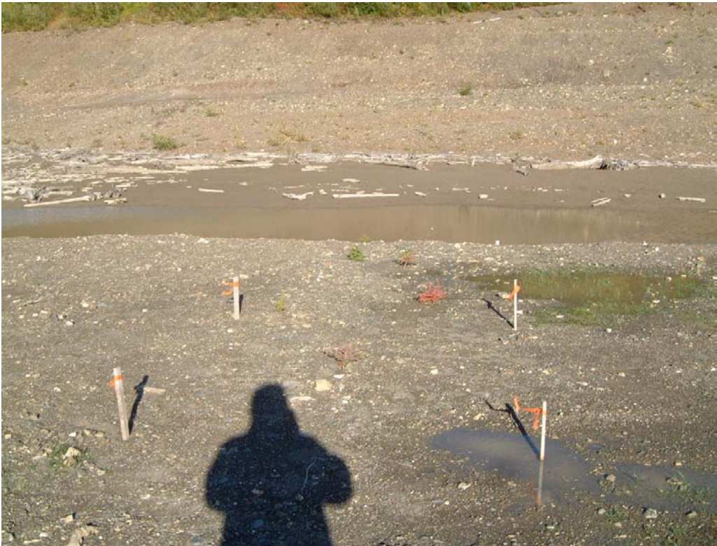
TMF with 500 mm rock and 300 mm soil – plot 3 in right foreground
