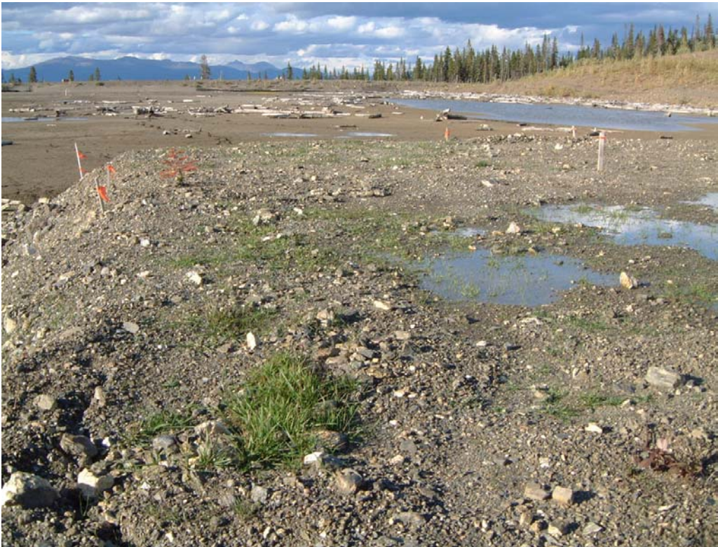
TMF with 500 mm rock and 300 mm soil – plot 1 in left foreground
