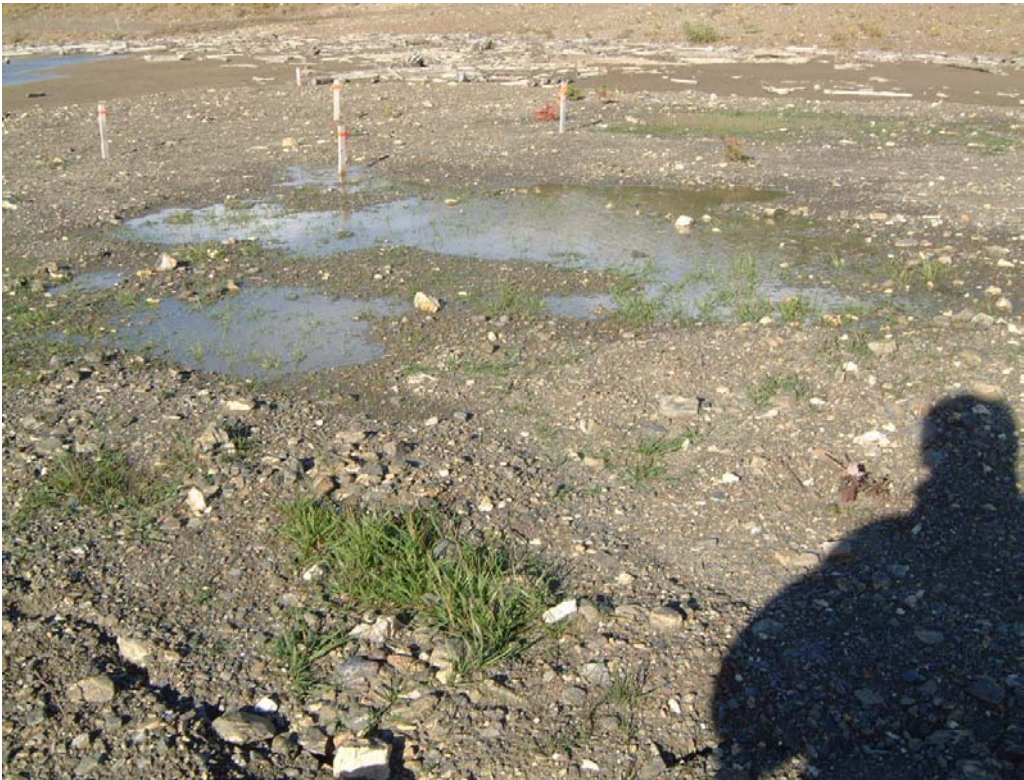
TMF with 500 mm rock and 300 mm soil – plot 1 in foreground
