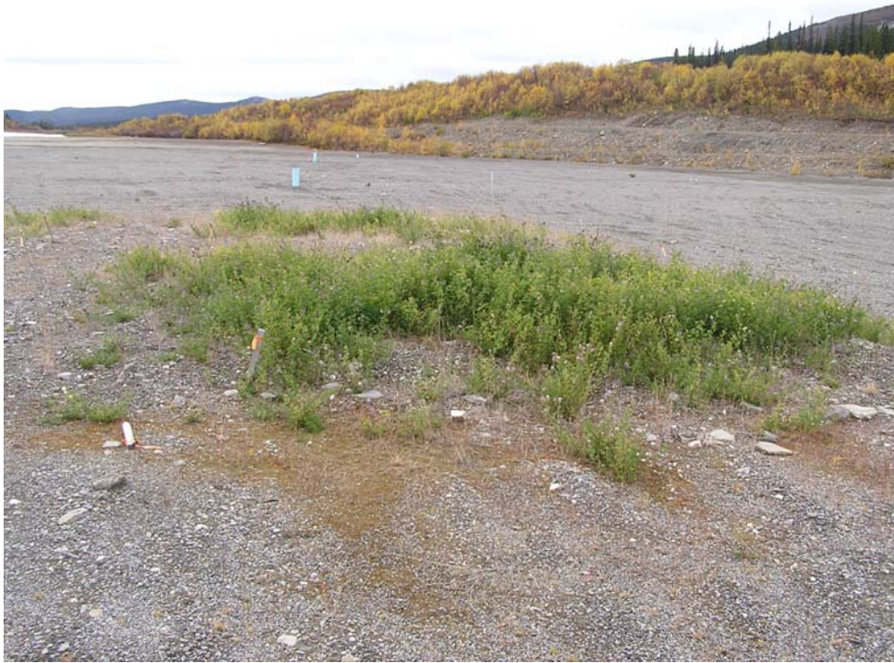
Site 5A Test Plots -TMF with 200 mm Soil (Note dense, patchy Alfalfa)
