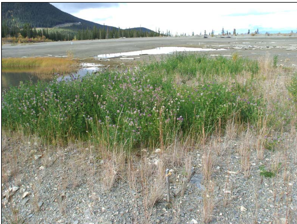
Site 5C Test Plots – TMF with 500 mm Rock and 300 mm Soil
