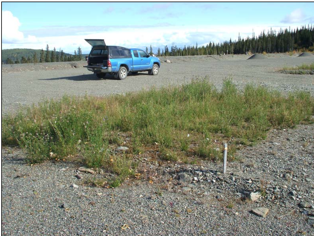
Site 5A Test Plots - TMF with 200 mm Soil (Note dense Alfalfa)
