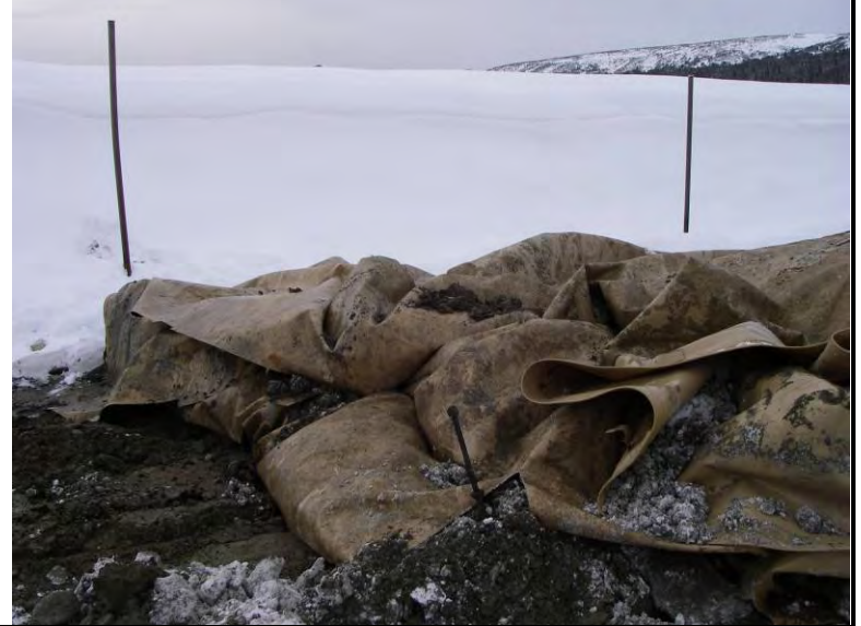
10/07/07 Tear in the middle of the berm from being pulled over
