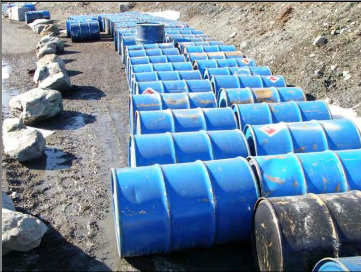
Photo 2. Arrangement of stored diesel drums in Cache A with spilled containers placed upright. The sealed drums are on their side to prevent contamination by rain water. Taken May 23, 2007.
