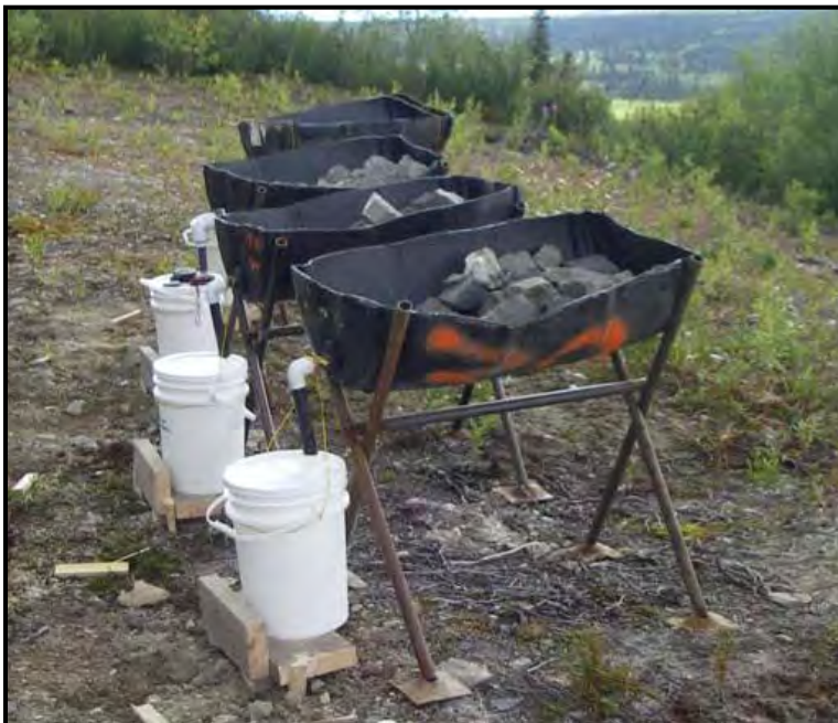
Picture 8-1: Wolverine Project Geochemical Test Pads
