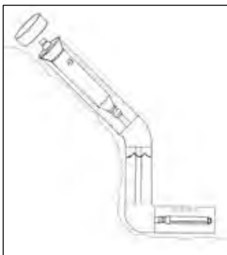
Figure 2-2: Flow Monitoring Level Logger Installation
