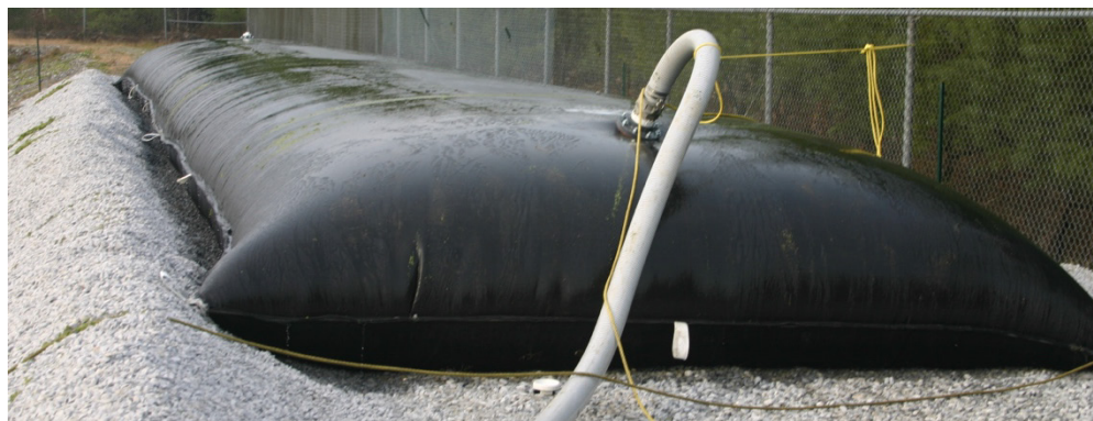
Photo 6-1: Example of a Geotube in Operation
