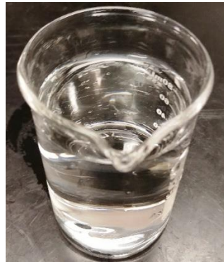
Figure 6-2 Effluent water from the metals removal stage. Solution is clear with no suspended solids.
