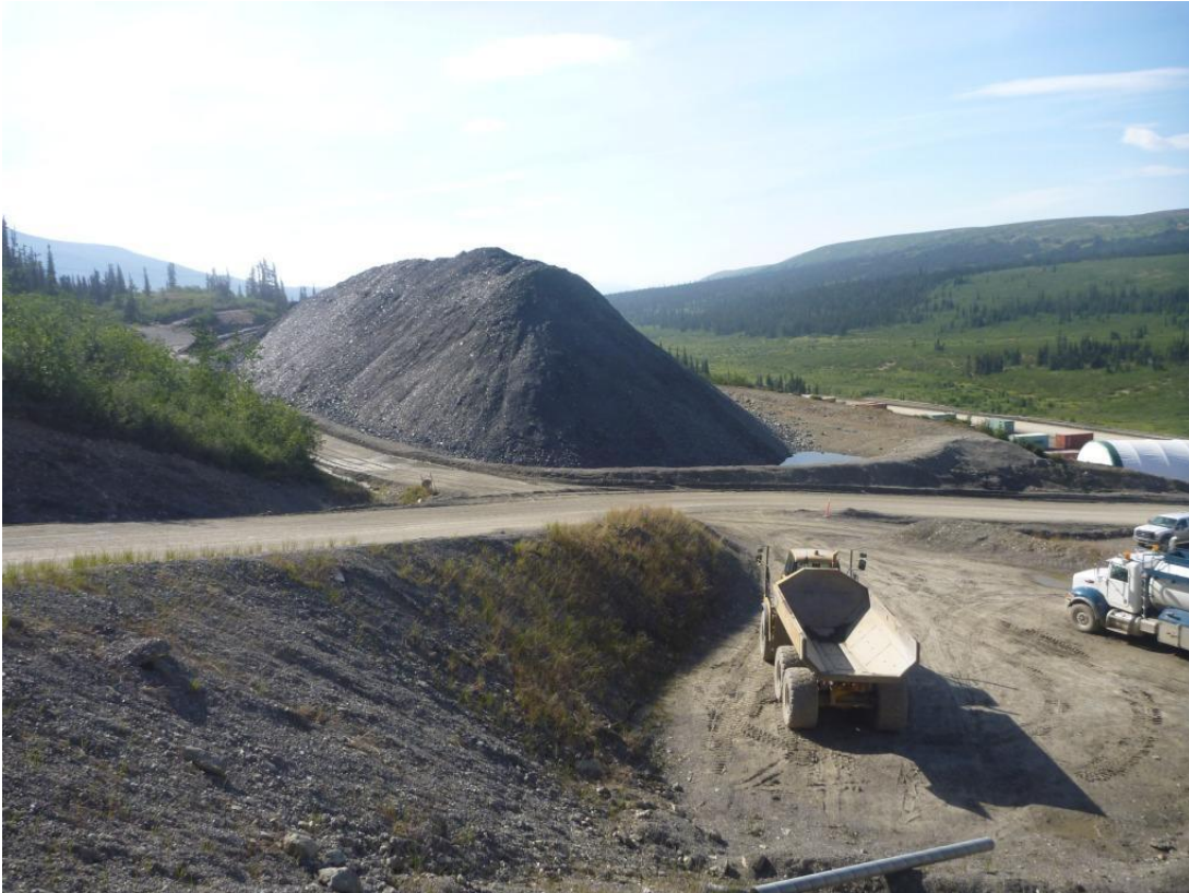
Picture 5-8: Test mine and pre-production waste rock on temporary waste rock storage pad located east of camp (July 14, 2013)
