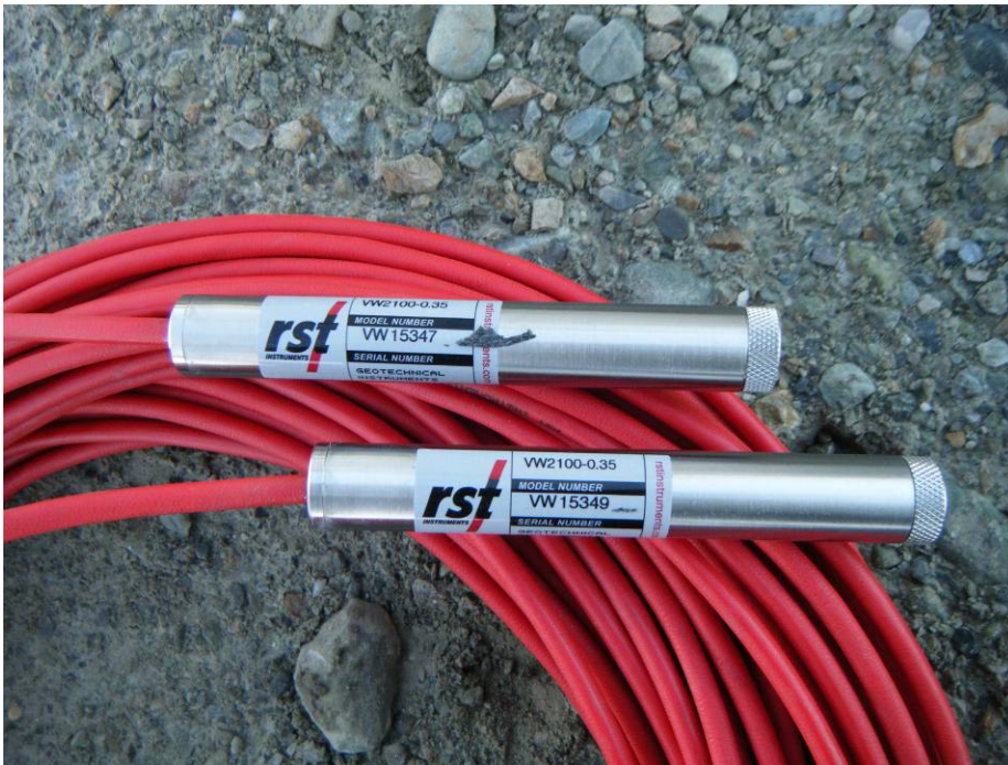
Photo 6 Vibrating Wire Piezometers
