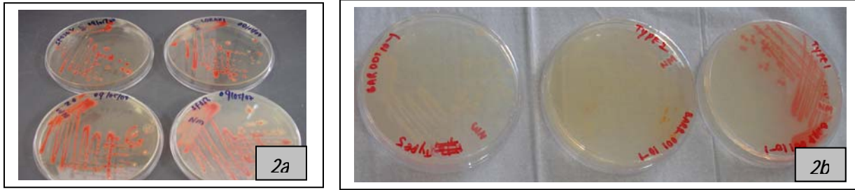
Figure 2a and 2b. 2a shows SF036, Z0, SF056, and Lorax-1 (L-1), the individual bioreactor test microbes, with good microbial growth and selenium reduction using a defined media. 2b shows a screen for selenium reduction using three different media containing different amounts of selected media components. The best growth and selenium reduction is on the plate on the right side of Figure 2b .
