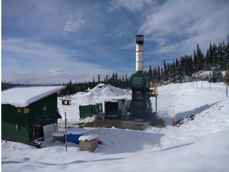
Picture 2-6: Incinerator (centre right) and ash storage bin (centre left) sitting on cement slab.
