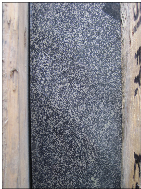
Net-textured sulphides in drill core, Wellgreen property.
