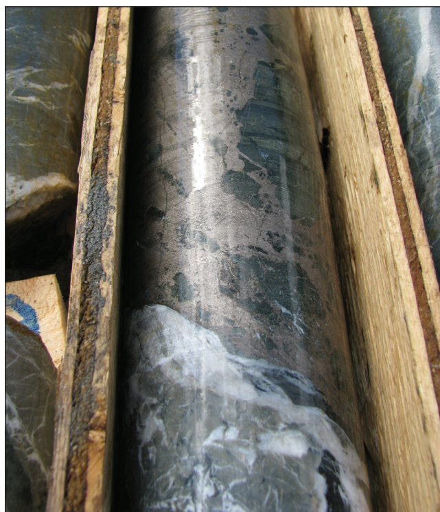
Massive pentlandite in drill core from the Nickel Shāw property, southwest Yukon.
