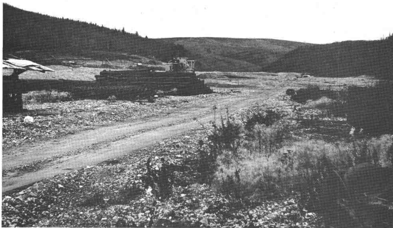
Figure 39 Placer gold mining operations in perennially frozen gravels in Bear Creek valley, a tributary of Klondike River near Dawson, Y.T. The stacks of pipe comprise the dismantled network through which cold water is circulated to thaw the frozen gravel. September 25, 1964.
