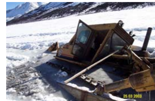
Saturated ground conditions 5
