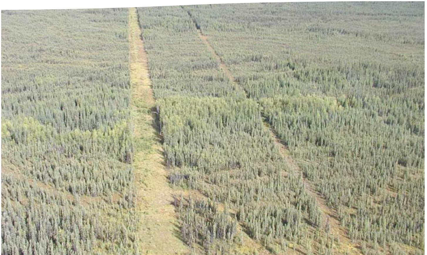
Conventional seismic line (5-8 m wide)
