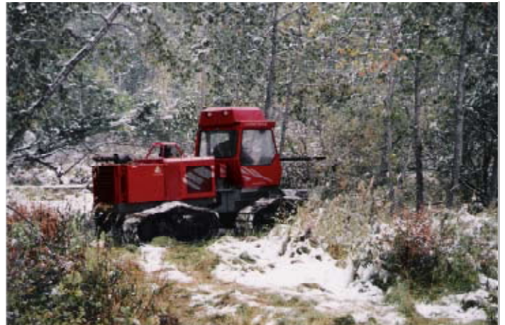
Light weight low ground pressure mulcher for narrow seismic lines, soft (muskeg) and hilly terrain fitted with 1.75 metre rotovator drum
