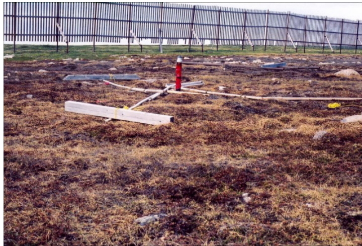
Figure 4.37: Photograph of Baker Lake BH2, looking away from the town and towards the snow fence (upwind). Note the brown vegetation from the long-lasting snow drift. Photo was taken on July 30, 2002, one week after the end of snowmelt (photo is courtesy of the Geological Survey of Canada).
