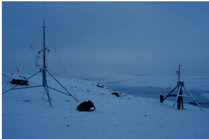
Figure 4.7: Photograph of weather station and borehole at Alert BH5, taken in August 2002 (photo is courtesy of the Geological Survey of Canada).
