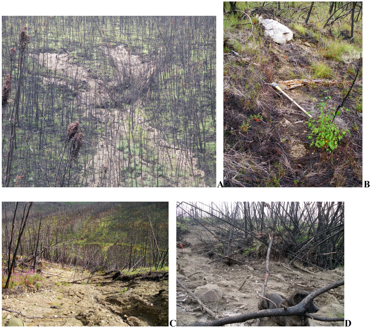
Figure 5.8: SC03 AB Photographs. A: View of failure from opposite slope showing extensive sediment plume development (July 2005). B: Tension gash near headscarp (August 16, 2005). C: Scar Floor looking downslope (July 20, 2006). D: Main displaced mass viewed from downslope (August 16, 2005).
