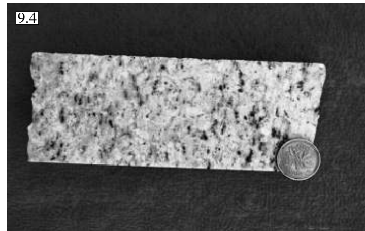
Figure 9 Felsite, aplite, and leucogranite samples. 9.1. Hand sample of massive felsite dyke material. Phenocrysts of quartz, feldspar, and biotite are visible in the aphanitic groundmass. 9.2. Photomicrograph of the felsite under crossed polars. 9.3. Hand sample of foliated aplite with small phenocrysts of biotite and magnetite. 9.4. Hand sample (00N-74) of leucogranite (alaskite?) with 5-10% biotite phenocrysts.
