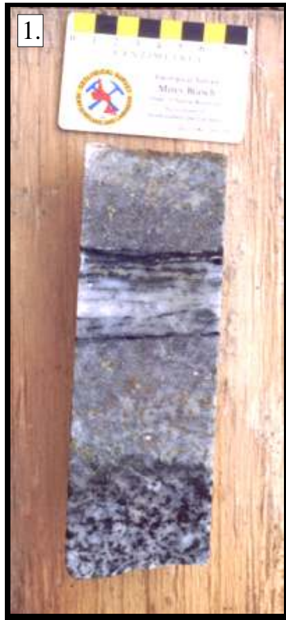
Figure 29 Alteration adjacent to the gold-bearing quartz veins. 1. Hand sample showing the banded texture in the vein (black bands are the tourmalinized wallrock slivers). The alteration envelope is 4-5 cm wide and consists of muscovite/sericite, pyrite, arsenopyrite, Fe-carbonate, and quartz. 2. Photomicrograph, under crossed polars, of the alteration envelope within 2 cm of the vein. Minerals present include quartz, pyrite (Py), arsenopyrite (Apy), bowtie-shaped muscovite after feldspars, muscovite/sericite pseudomorphs after hornblende and biotite, and in the fine-grained groundmass there is sericite and carbonate.
