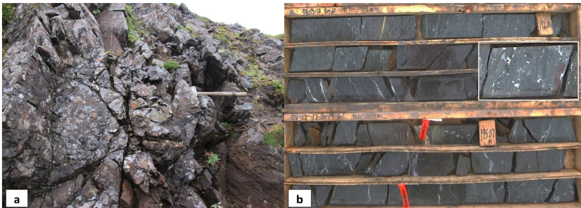
Figure 3.5 A., Mafic volcanic breccia in outcrop. B., Mafic volcanic breccia with chlorite-rich matrix in drill core.
