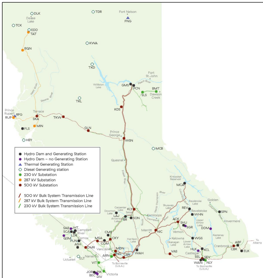
Figure 2.5: BC Transmission System
