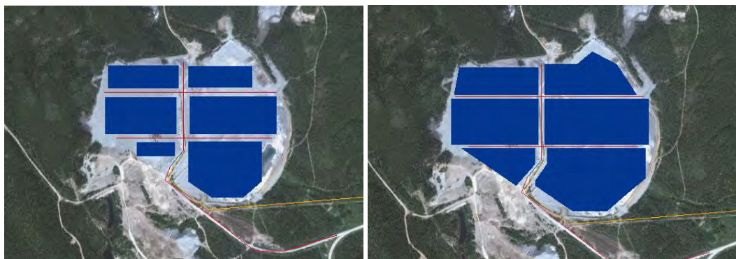
Figure 9.5: 10 MW fixed tilt area requirements at Whitehorse. Left: Smallest (80 acres); Right: Largest (107 acres)
