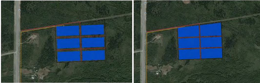
Figure 8.3: 5 MW fixed tilt area requirements at Haines Junction. Left: Smallest (40 acres); Right: Largest (53.6 acres)
