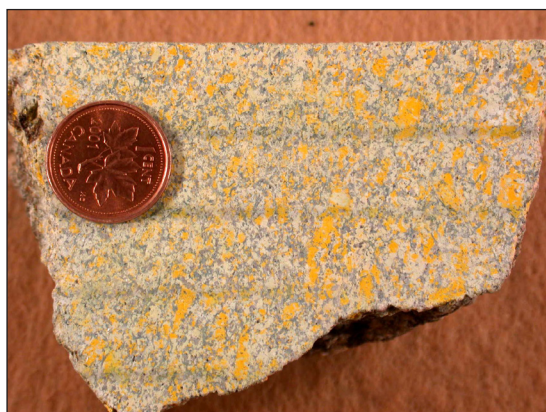
Figure 13. Slab of Anvil plutonic suite muscovite-biotite granite. Stained for K-feldspar. Penny is 1.9 cm across. Field station 84-50. Photo from Pigage (2004).
