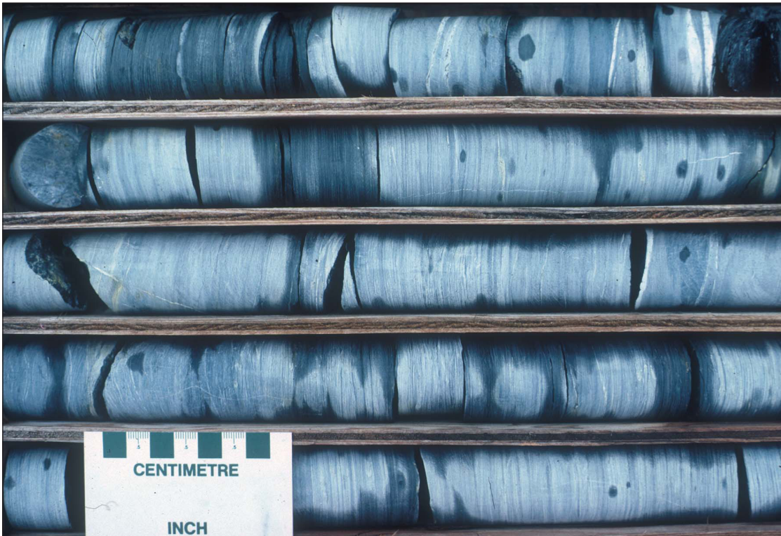
Figure 4. Muscovite-chlorite phyllite of the Mount Mye formation. BQ size core from drill hole CNR76-01 (130-137 m). Photo from Pigage (2004).
