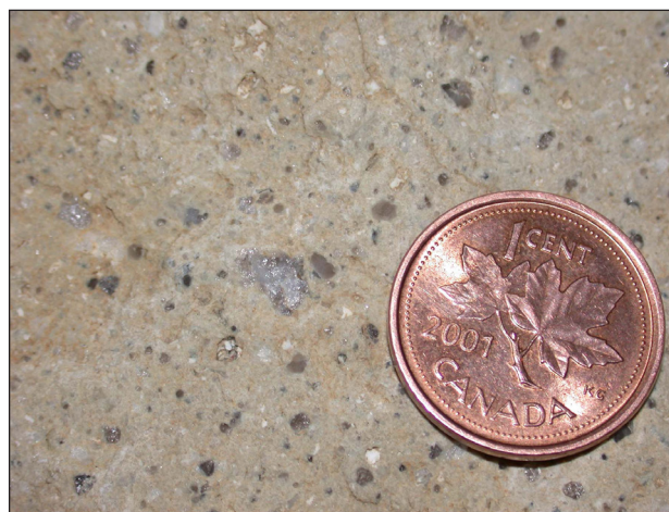
Figure 16. Eocene quartz-feldspar porphyry. Smokey quartz and small white feldspar phenocrysts. Sample from northeast wall of Faro open pit. Penny is 1.9 cm across. Photo from Pigage (2004).
