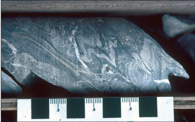
Figure 17. D1 minor fold defined by siltstone bed in Vangorda formation. Drill hole 76X-11 (22 m). NQ size core. Photo from Pigage (2004).
