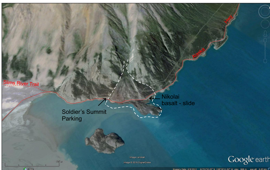
Figure 3-12. Google Earth image of southern Kluane Lake showing the distribution of slide rock near Soldier's Summit. The slide is composed entirely of basalt of the Triassic Nikolai formation (Stop 3-1).
