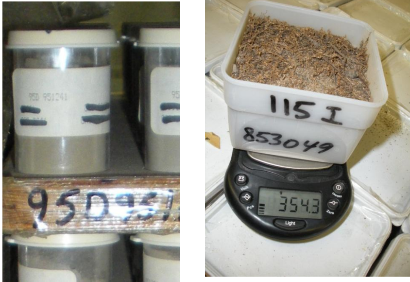
Photos 1 and 2. Photos showing ball-milled stream sediment pulps stored in vials and raw (unprocessed) steam sediment sorted in freezettes.
