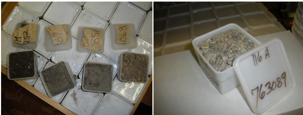
Photos 3 and 4. Photos showing examples of saved raw samples that range from fine to coarse grained material. The darker sample on the far left indicates some organic content.
