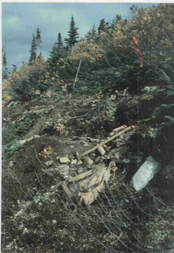
Two hand-dug pits @ 100 meters east of discovery gully. Bedrock in pits exposes low-grade, base metal sulfides in schist. Sleeper Claim No. 9
