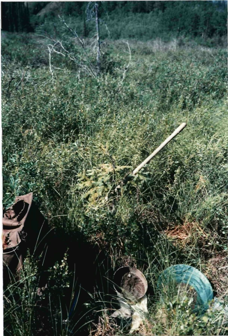
Test Pit for Sampling of Moraine Till
