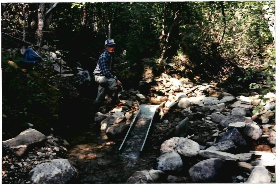
Trench material being sluiced in Target # 1 creek. Trench is behind me.
