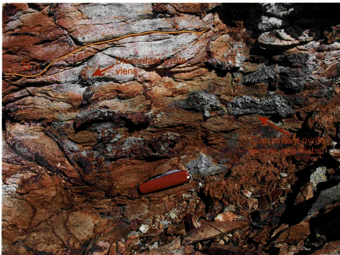
Plate 2 - Close-up of characteristic mineralization in the quartz-sericite altered tuffs. Both concordant cm-scale lenses and discordant pyrite mineralized veins are depicted.
