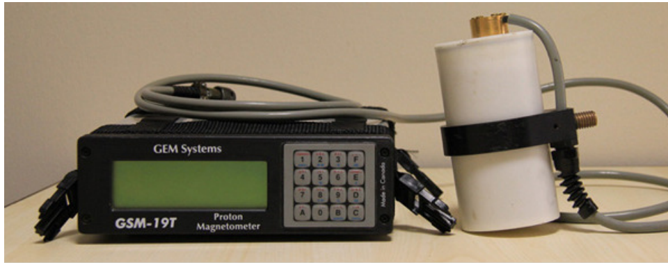
Figure 12: GEM GSM-19T proton precession magnetometer.
