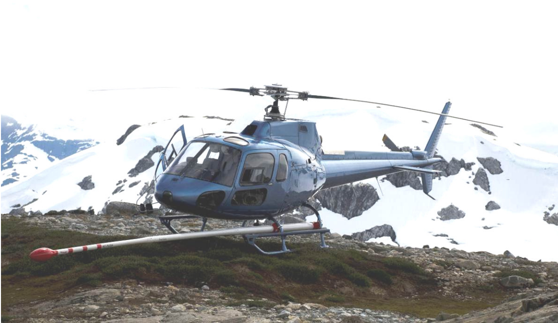
Figure 8: Eurocopter AS350 equipped with mag stinger for magnetic data acquisition, and internal spectrometer crystals for radiometric data acquisition.
