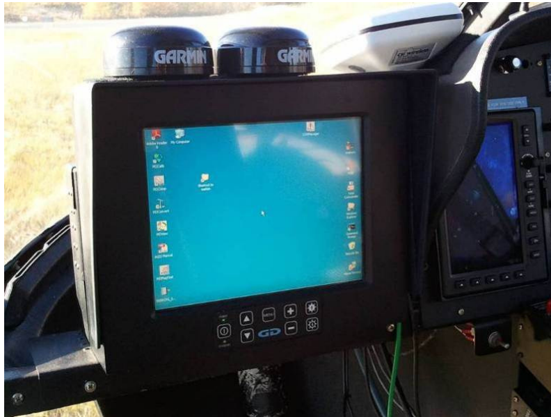
Figure 9: AGIS installed in the Eurocopter AS350.
