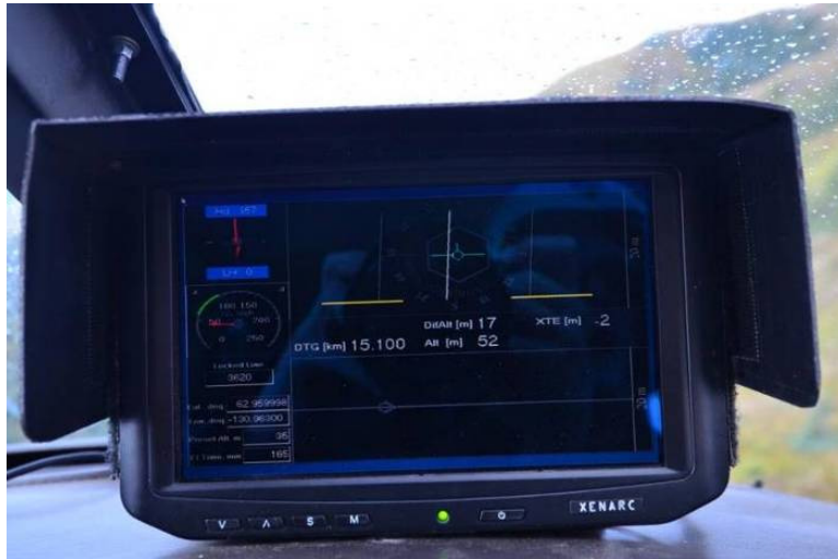
Figure14: Pilot Guidance Unit.
