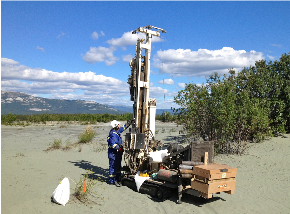
Figure 7. Sonic Drilling, view west over Grey Mountain from Tailings Ponds, July 2013
