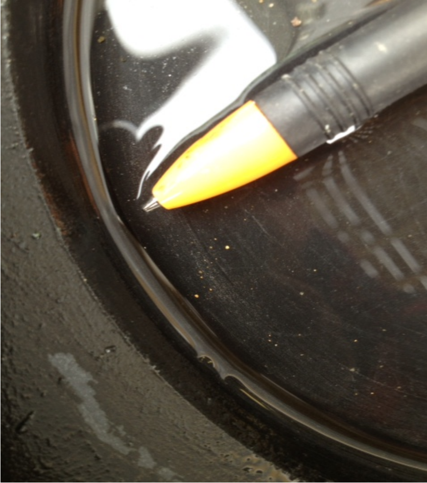
Figure 8. Fine gold particles recovered from 2013 samples.
