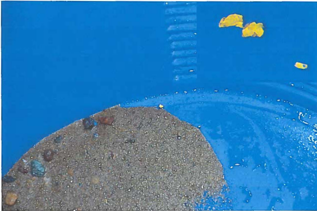
Plate 7 - Concentrates from BD Pit 3 consisted of fine pyrite and coarse garnet and ilmenite. Inset photo - gold colours were "chunky" and not flat. The larger grains are approximately 1.2 mm across.
