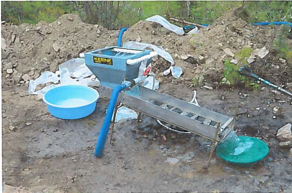
Plate 6 - Drill samples were processed in the field using a Keene A52 sluicebox.
