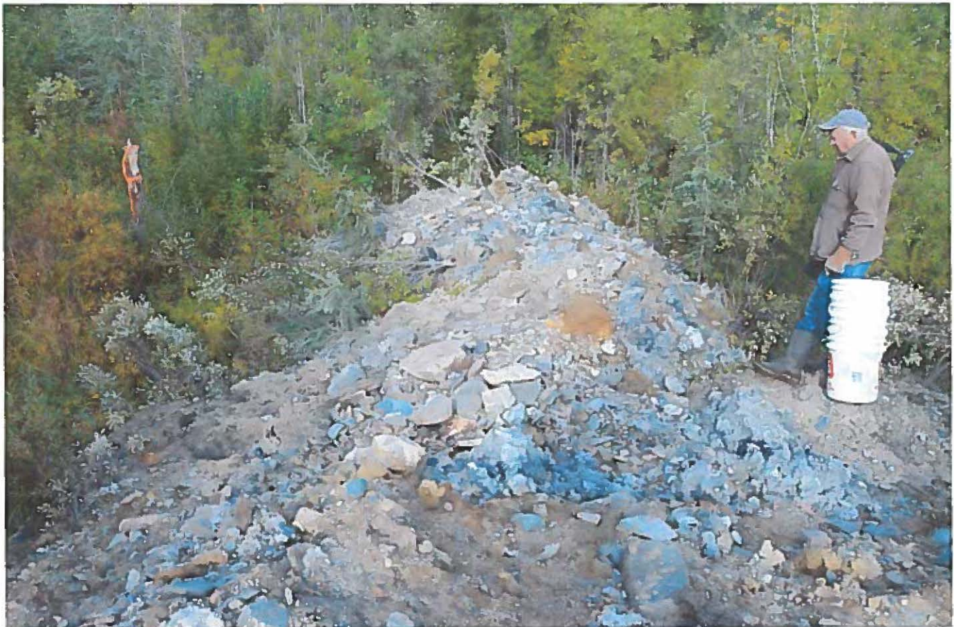
Plate 5 - Excavator test pit BD Pit 3 reached clay-altered bedrock at a depth of 5 metres adjacent to the Queenstake pit. Material was stockpiled for sampling.
