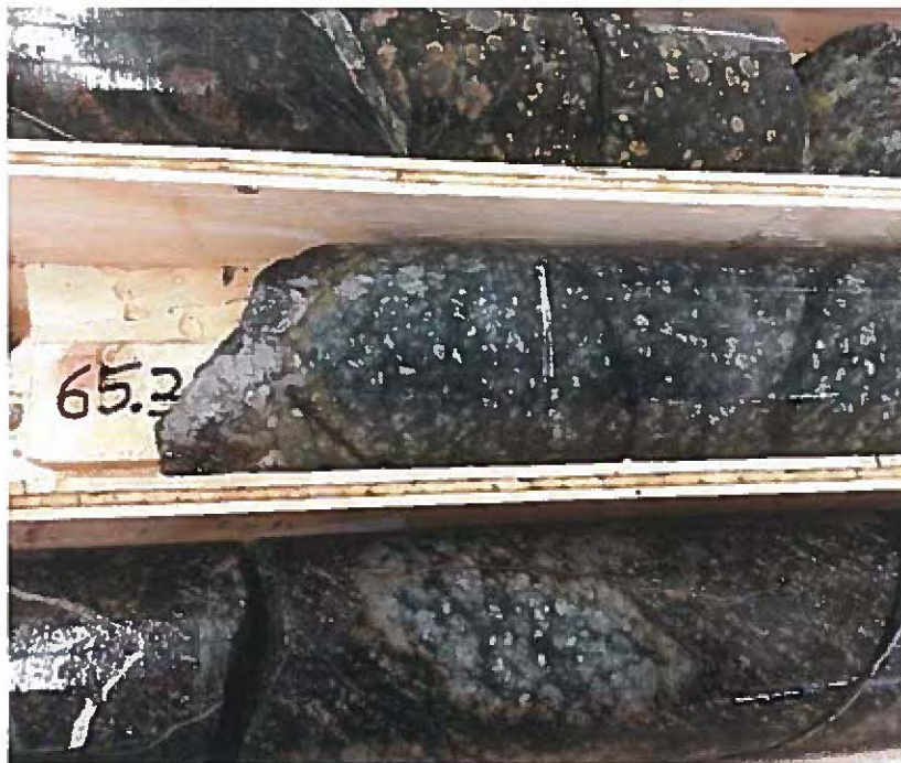
Fig. 24: Variable textures in drill hole 1, 64 to 66 m depth of HTW core (71mm diameter) upper row of spheroidal texture with altered rims of dunite fragments, crackled peridotite in the middle row and lower
