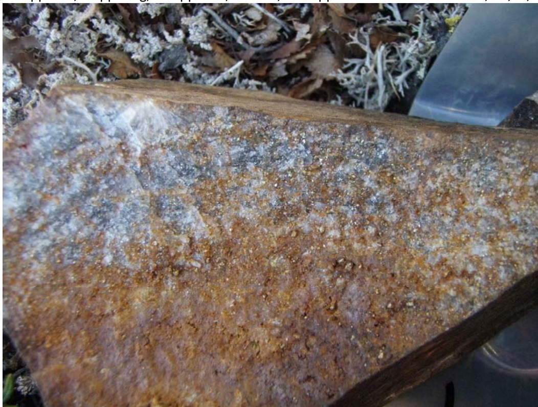
Photo 3: Rock sample 1768021 from the North Zone. Pyrite-rich quartzite yielding 643 ppm Au, 37 ppm As, and 3524 ppm Cu (sample is about 5" across).
