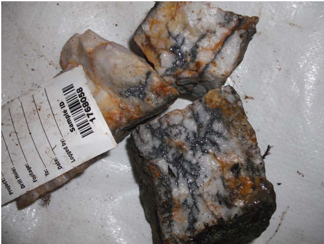
Photo 2: Rock sample 1768058 from the Main Zone. Galena and pyrite mineralization in quartz vein yielding 231 ppb Au, 57 ppm Ag, 225 ppm As, >1% Pb, >100 ppm Se and anomalous Mo, Cu, Bi, Hg, Te.
