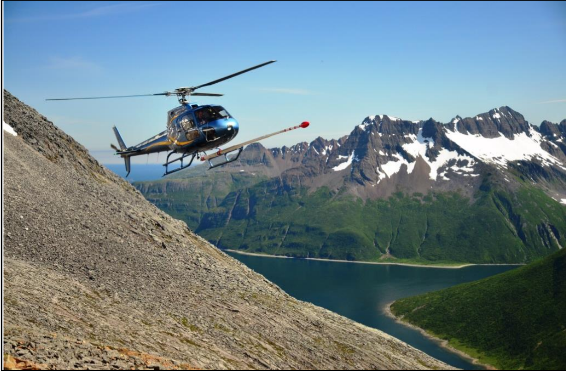
Figure 10: Eurocopter AS350 helicopter equipped with mag stinger for magnetic data acquisition, and internal spectrometer crystals for radiometric data acquisition.
